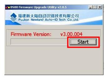
Step 5: Connect the scanner to your PC with the USB cable. Then the update begins. The red and blue Function LEDs flash alternately during the updating process.
