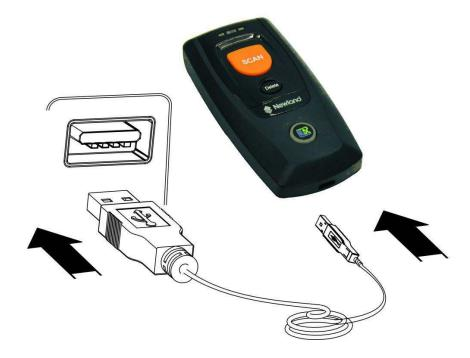
Note: Low battery may result in failure or misoperation of the scanner. Before your first use, charge the battery for 3-4 hours.
