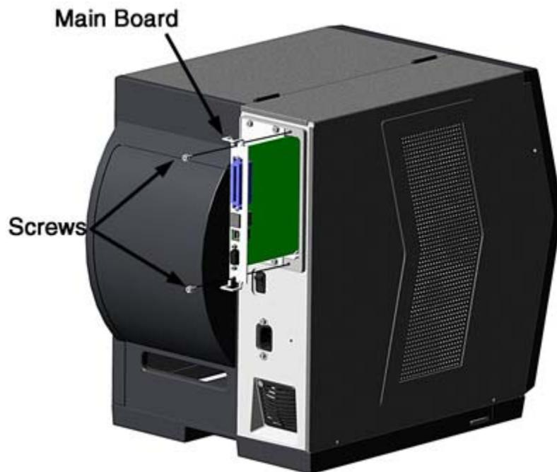
4. Slide the Main Board out of the printer then move the jumpers according the needs of the application:
