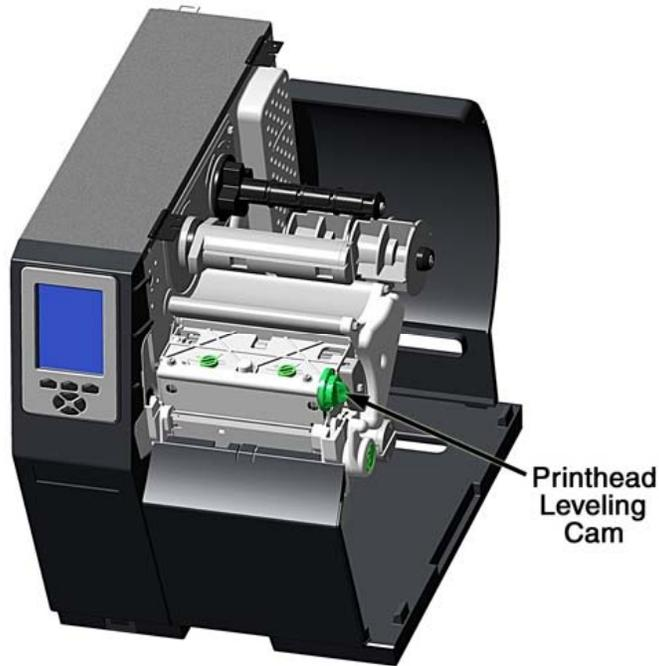
Adjust the Printhead Leveling Cam as follows:
